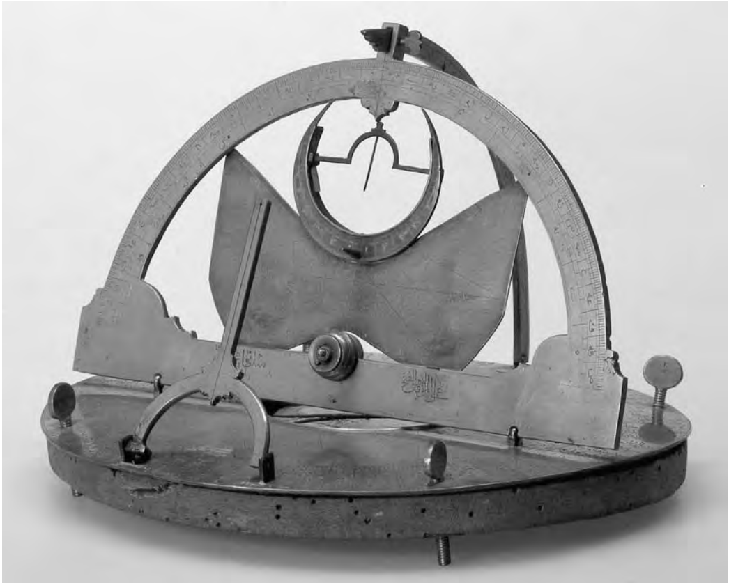
[iv] Qibla compass and sundial, open: Istanbul, 1161/1748. This complex device, termed an “equatorial circle” ( dār al-mu'addil ) by its ninth/fifteenth century Egyptian inventor, combines a qibla compass with a sundial. Courtesy of the Nasser D. Khalili Collection, London (SCI 270).
